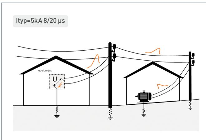
The lifetime is described by the number of hits that **the SPD is able to withstand at Typical Surge Current ( $I_{typ}$ )**.
