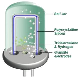
The TCS is then sent to the CVD (Chemical Vapor Deposition) reactor. In the Siemens process, high-purity silicon "starter" rods or hairpins are exposed to trichlorosilane at 1150 °C in the CVD reactor. The trichlorosilane gas decomposes and deposits additional pure silicon onto the rods in the CVD reactor, enlarging them according to chemical reactions like:
